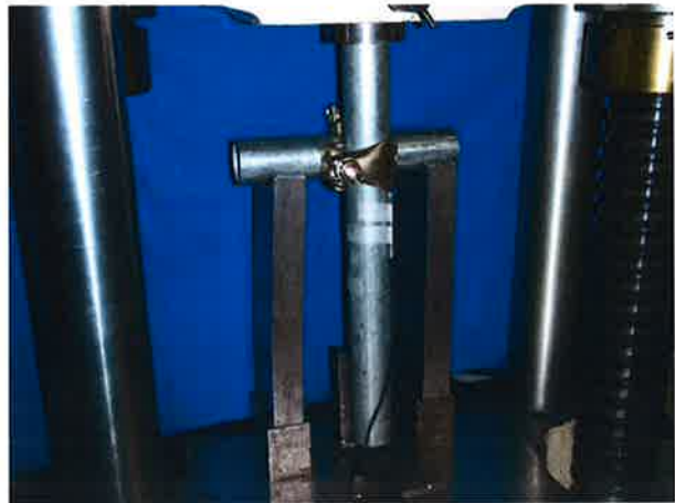
Photograph of Setup for Slipping Force
